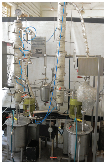
Closed-loop absorber-desorber setup for CO 2 capture using alkanolamines
