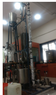
Thermal Hydraulic Studies on Boiling in Vertical Tubes
