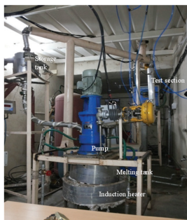
Figure 2: Molten salt flow loop
