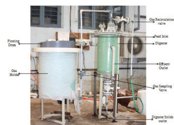
Figure 3: Bio gas generation from food waste
